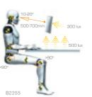
The new Forward Arm puts the user in control of the screen position, ensuring optimum workstation ergonomics and maximum working comfort. *Tip:* make sure that you are one arm's distance from your screen.
